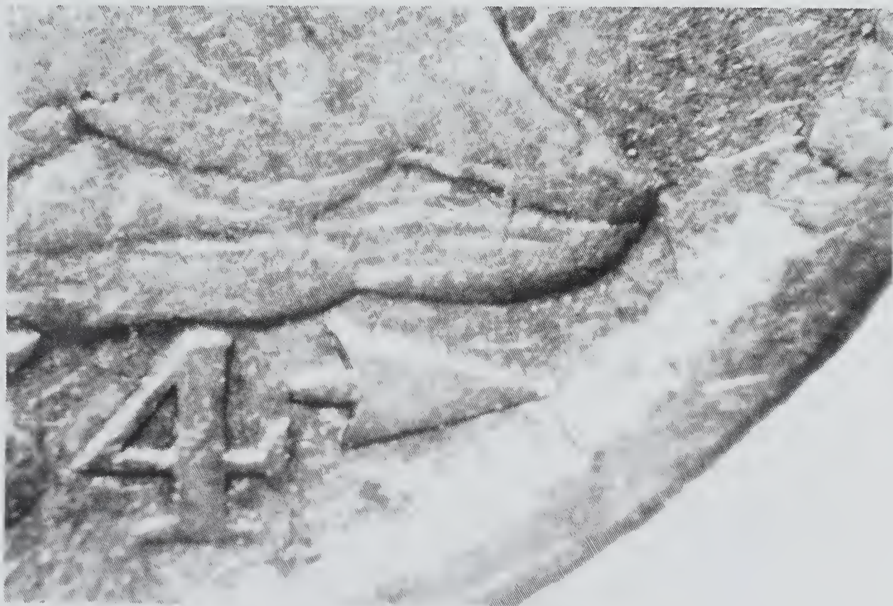
Late Die State 1854-O V-1 Half Dime with Die File Line through Foot
