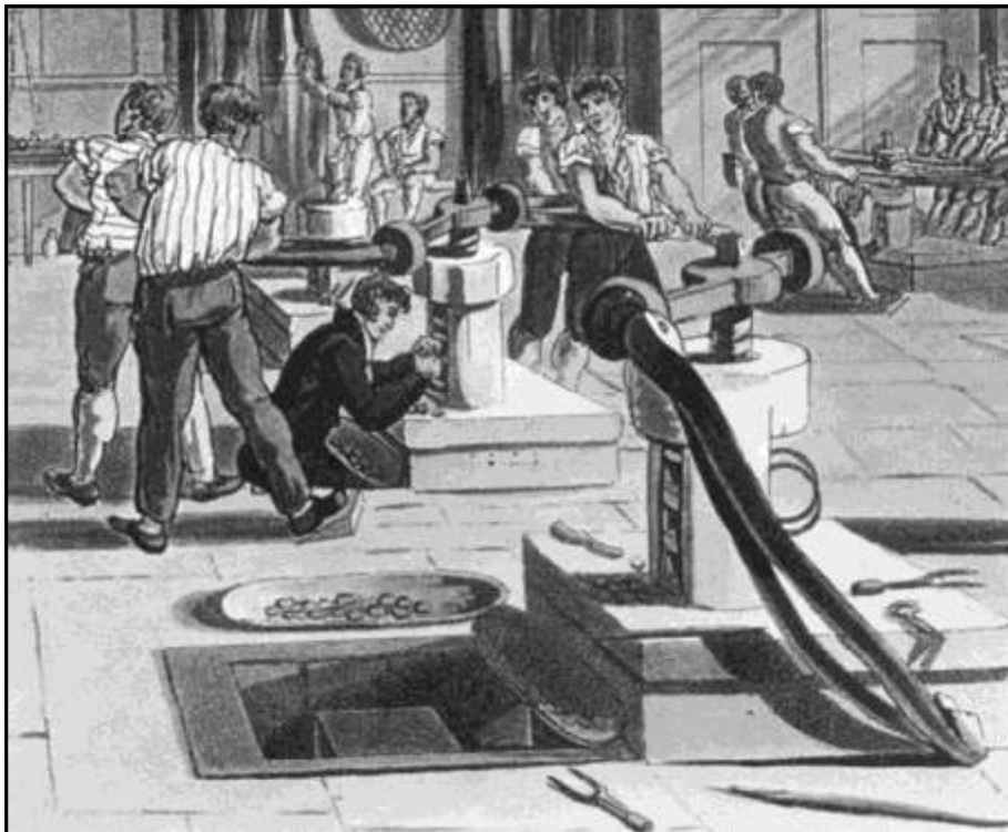
Figure 1. Tower Mint screw presses from Ackermann's "Microcosm of London" circa 1811. (Continued on next page)
