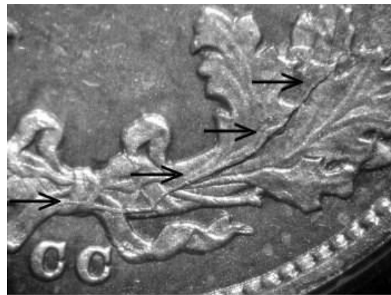
Die crack through lower right wreath
