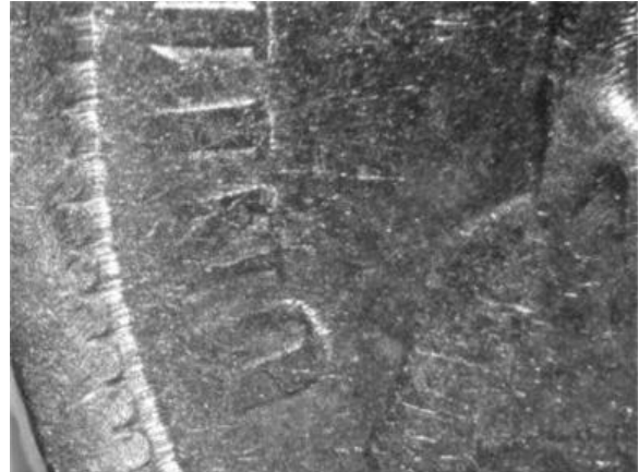
Obverse 2 - Late Die State Severe die erosion at (UNIT)ED
