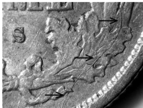
Reverse D Lower right wreath die crack through right ribbon end
