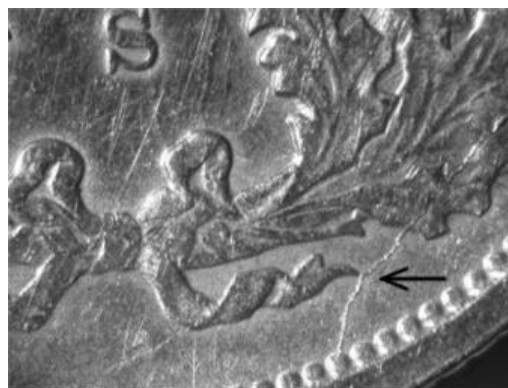
Reverse C Lower right wreath die crack touches right ribbon end
