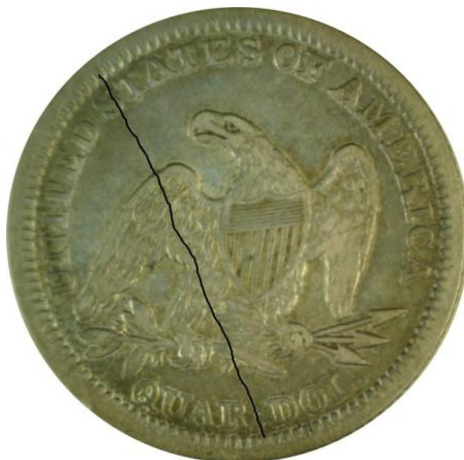
1845 Quarter Dollar– reverse die crack
