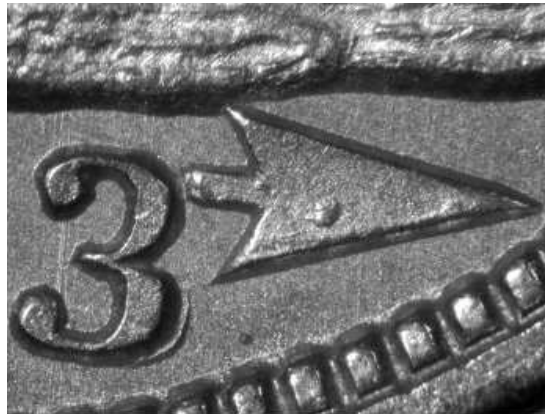
Die defect on right arrow
