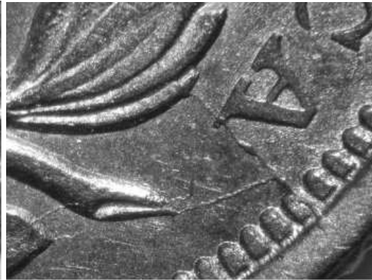
Die cracks from lower right wreath to rim
