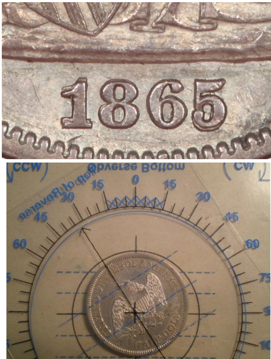
Rota-Flip Die Rotation Device measuring the reverse of an 1865/1865 half dollar
