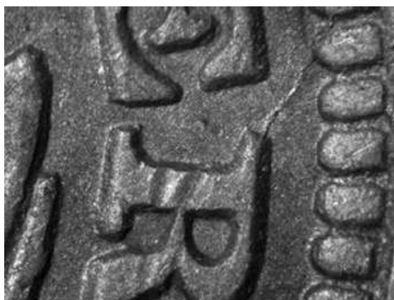
Die crack from rim to AME(R)ICA
