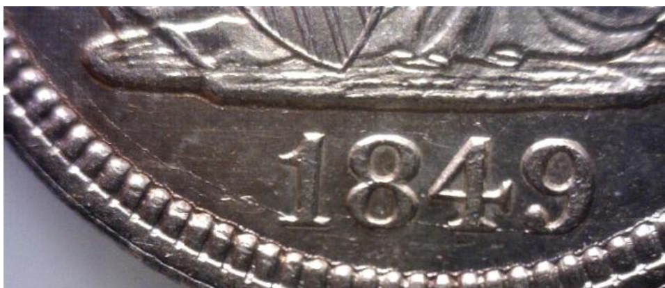
Figure 3. 1849 Quarter Obverse 3 – Die Crack Close Up
