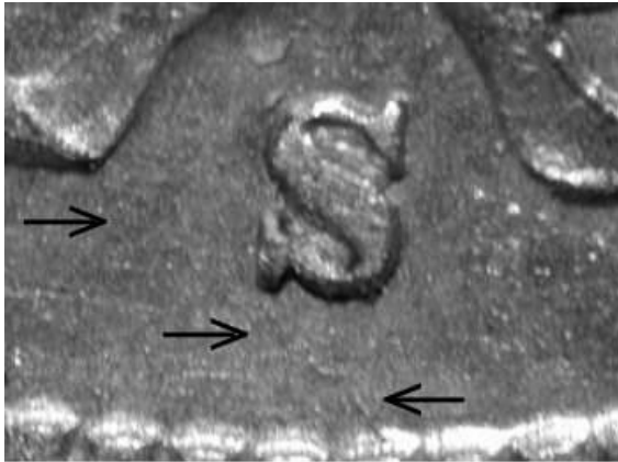
Die crack from left ribbon to rim
