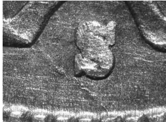
Die crack from left ribbon to rim
