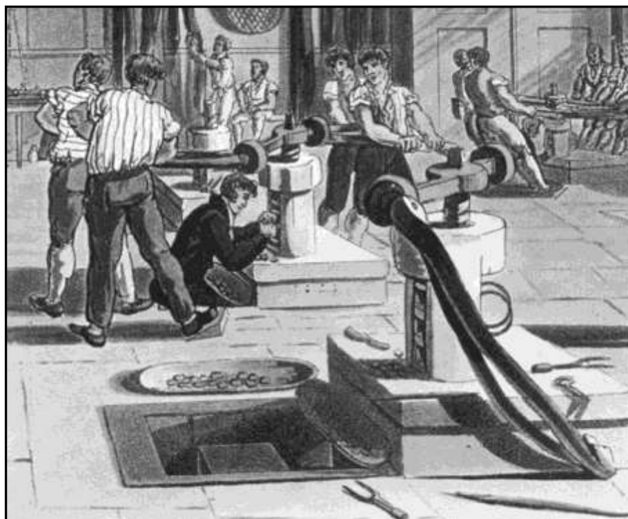
Figure 1. Tower Mint screw presses from Ackermann's "Microcosm of London" circa 1811.
