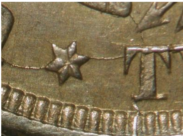
Die Cracks at and around TWENTY
