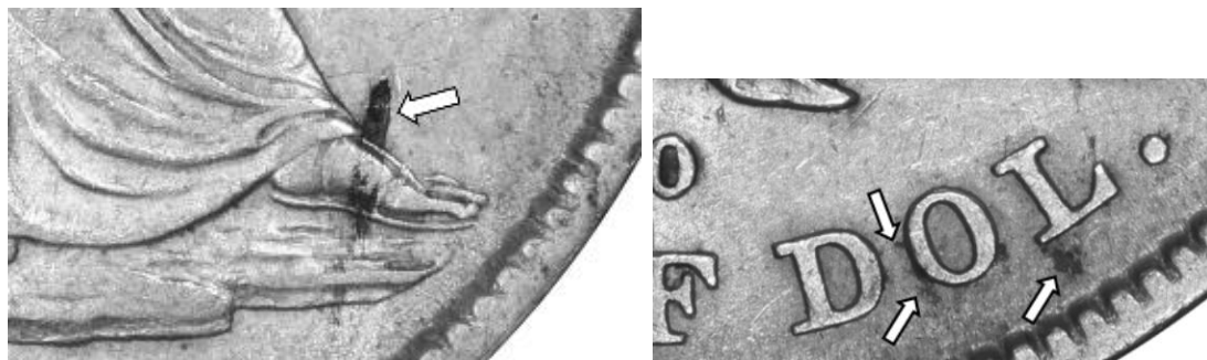
Iron bits in the planchet of an 1840-O WB-10 half dollar
