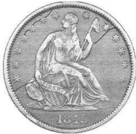
Obverse 5 (enhanced die cracks in photo at right)
